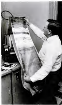
RECORDING SIGNALS at an RCA office in New York. Joseph Unger checks machine used to translate radio sounds into lines on a long roll of paper.
